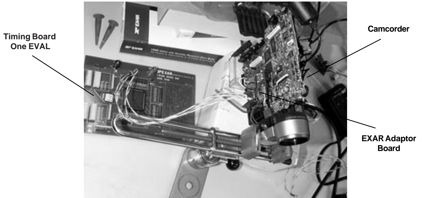
Figure 3. Timing Board One EVAL (Serial Port Programming Board, Ordered Separately) Connected to the Exar Adaptor Board Which Programs the Serial Port of the XRD98L59
